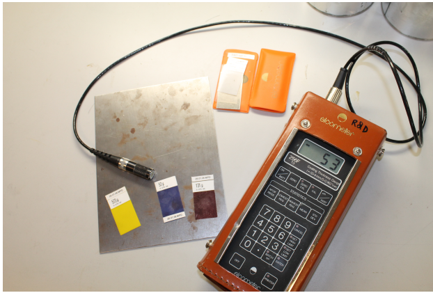
Figure 14.1: Elcometer 355 magnetic gauge, with coating thickness standards.
