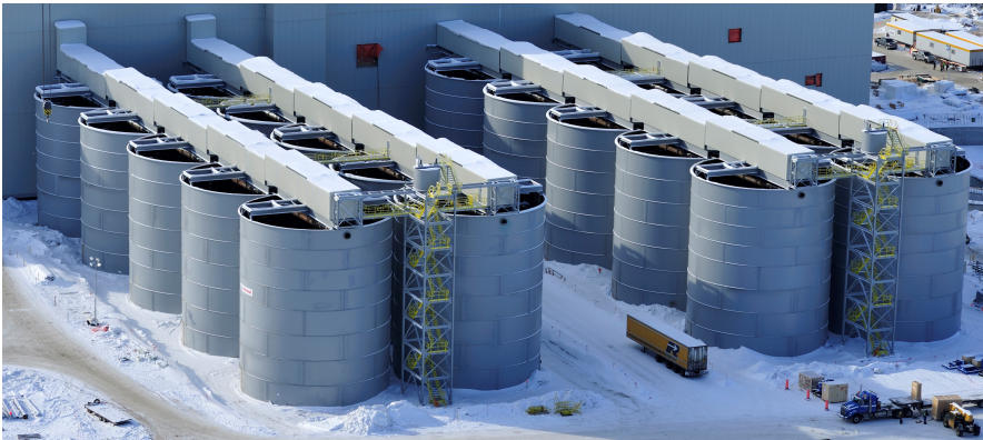
Figure 15.1: A series of industrial scale agitated leaching tanks for processing mineral ore, located in Cochrane, Ontario, Canada. Courtesy and copyright Fournier Industries. Observe the truck in the bottom right hand corner for scale.
