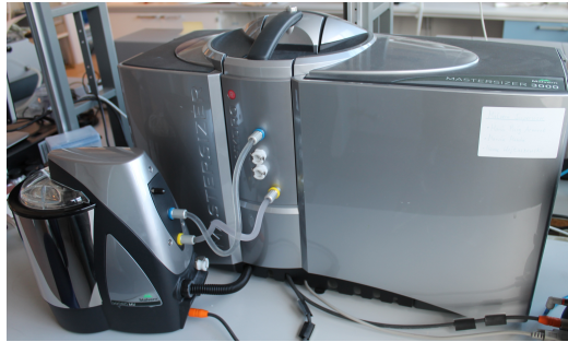
Figure 14.2: Malvern Mastersizer 3000 with liquid dispersion attachment. Capable of determining PSD using laser defraction.
