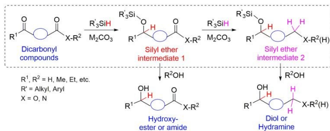
Fig. 1. Selective hydrogenation of dicarbonyl compounds to hydroxy-ester/amide or diol/hydramine catalysed by alkali carbonates ( M_2CO_3 ).
