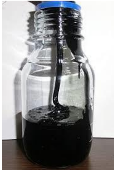
Plate 4. Heavy fuel oil. Before combustion it is heated in order to achieve a suitable viscosity
