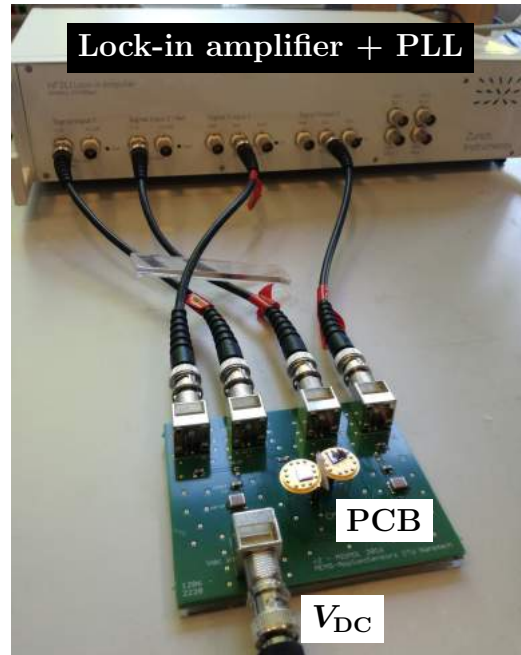
Figure 5.17: Photograph of the custom made PCB connected to a DC voltage supply (not shown) and the lock-in amplifier containing the PLL. The coaxial cables shown have a length of 0.25 m.
