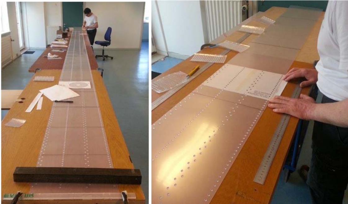
Figure 9 - Adding spacers (bump-ons) and lining up spiral windings (black lines)
