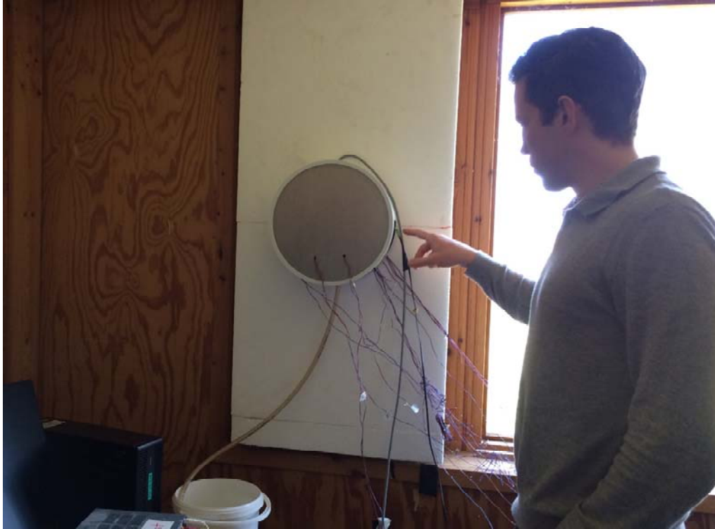
Figure 23 - Spiralflow unit attached with thermocouples to measure its heat exchanging efficiency.
