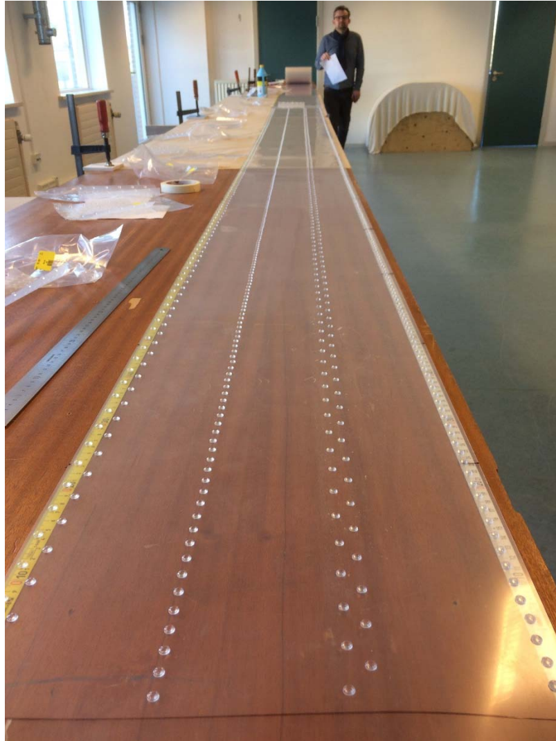
Figure 5 - Placements of the bump-ons on the plastic foil, before the heat exchanger is rolled up.
