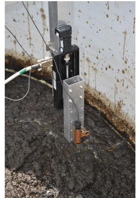
(d). The microsensor fixed to the micromanipulator.
