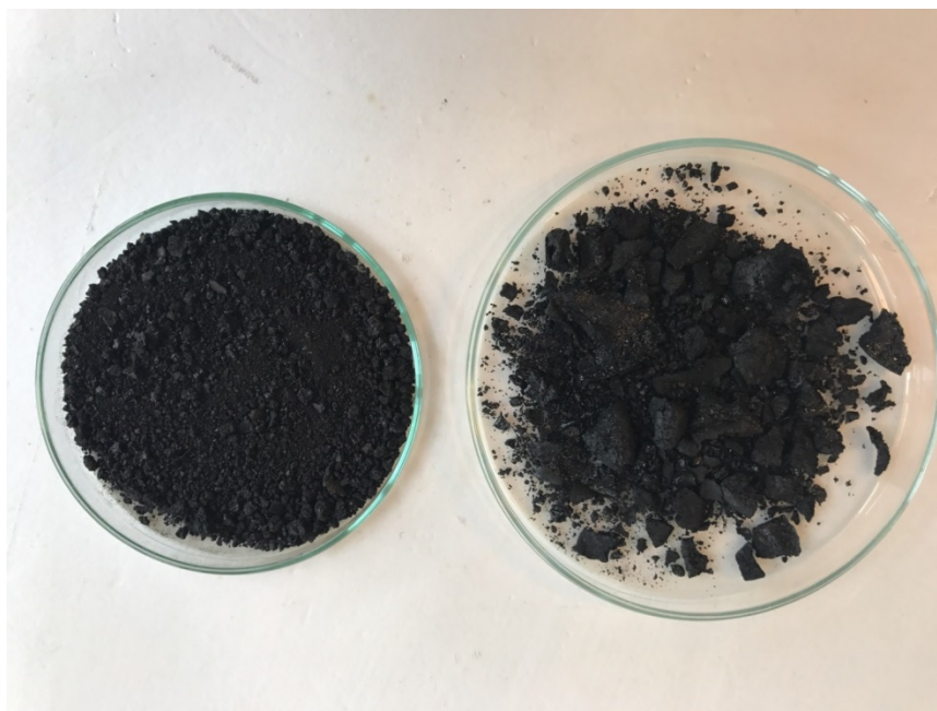
Figure B3 The physical appearance of the solid fractions from non-catalytic and catalytic conversion of H-LS at 310 °C (Table 13, Entry 1 & 2). (Right): Non catalytic solid, (Left): Catalytic solid. Reaction condition: 0/1 g catalyst: 10 g lignin: 100 ml solvent, 26 bar H 2 (loaded at RT), 3 hours.
