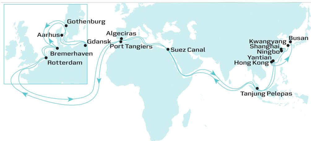
**Fig. 3** The Asia-Europe Service (AE10) from the 2016 Maersk Line Network. The round trip takes 12 weeks; hence 12 vessels are deployed to the service to ensure weekly departures. *Picture: Maersk Line.*
