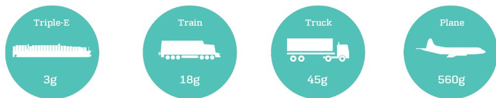
**Fig. 1** Grams of CO<sub>2</sub> emitted by transporting 1 tonne of cargo 1 km, using respectively container vessels, trains, trucks or planes. (Source: Maersk, 2015)
