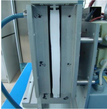
Figure 3(a): Side View of MD Cassette [28] Figure 3(b): PTFE Membrane Cassette inside module [28]
