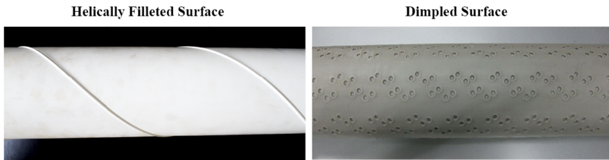
Figure 3.1 - Cable sample models from previous aerodynamic measures.
