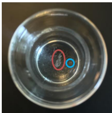
Figure 6.1. Photograph of separate crystals formed from crystallising product (highlighted in blue) in the presence of an externally added substrate crystal (circled in red).
