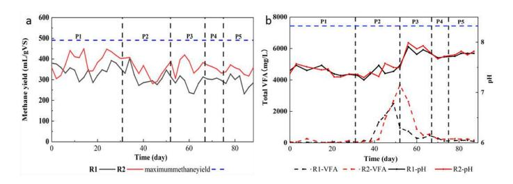
Figure 1.1 a) Methane yield and TAN change, b) VFA and pH variation throughout the experimental period
