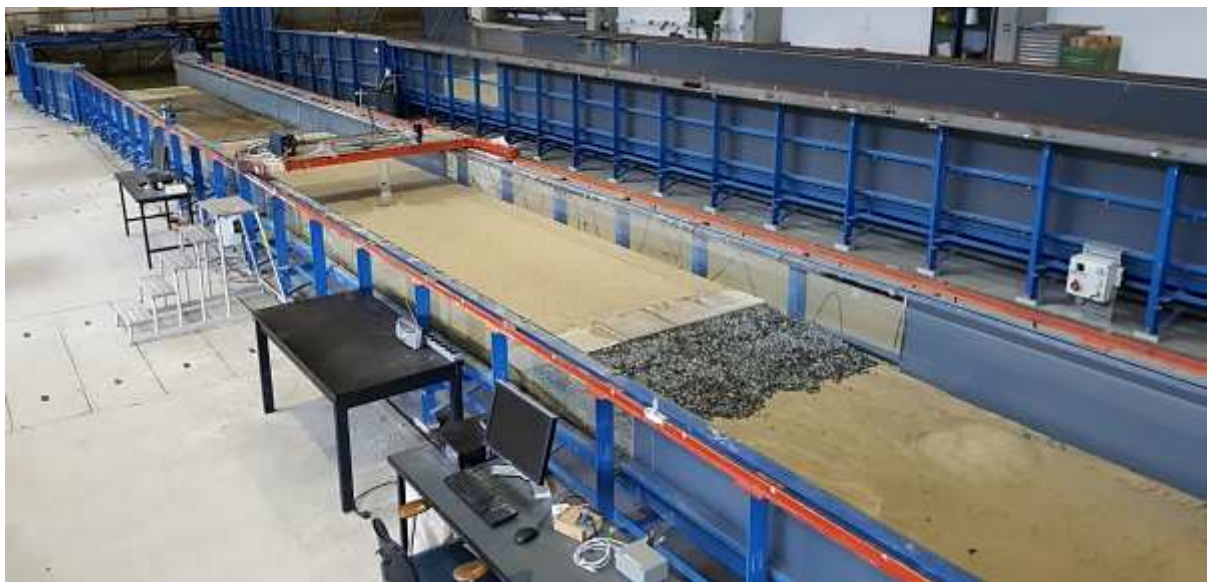
Figure 2: An image of the set-up in the flume. The carriage used when recording the bed topology is in this image over the upstream end of the sand bed.
