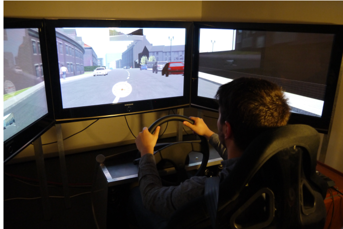
Figure 3.5: The driving simulator set-up.
