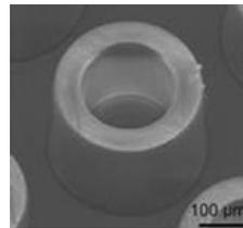
Figure 1: SEM image of a SU-8 microcontainer
