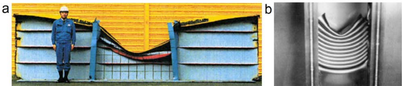
Fig 4: (a) Folding and (b) concertina tearing of web girders under local in-plane loads; cf. Refs. [19, 20].
