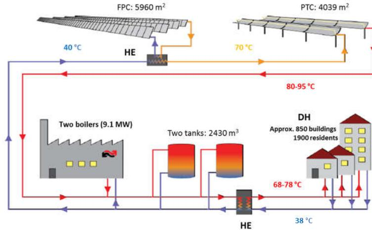
Fig.2. Schematic illustration of Taars solar heating plant.
