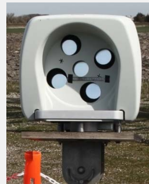
Avent 5-beam Demonstrator (5B-Demo): pulsed, step-staring
