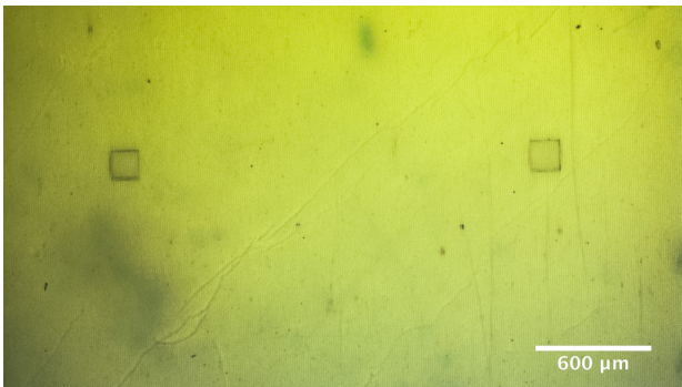
Figure 7. Optical microscope image of two square fiducial markers.
