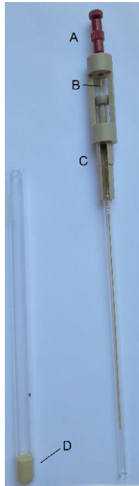
Figure 21 Flow cell with A) PEEK top with adaptors for tubes B) GC-tube centered in the NMR tube C) the top can be placed on a 5 or 10 mm tube D) a 10 mm tube with a PEEK plug to reduce the dead volume of the tube and ensure homogeneous flow through cells.
