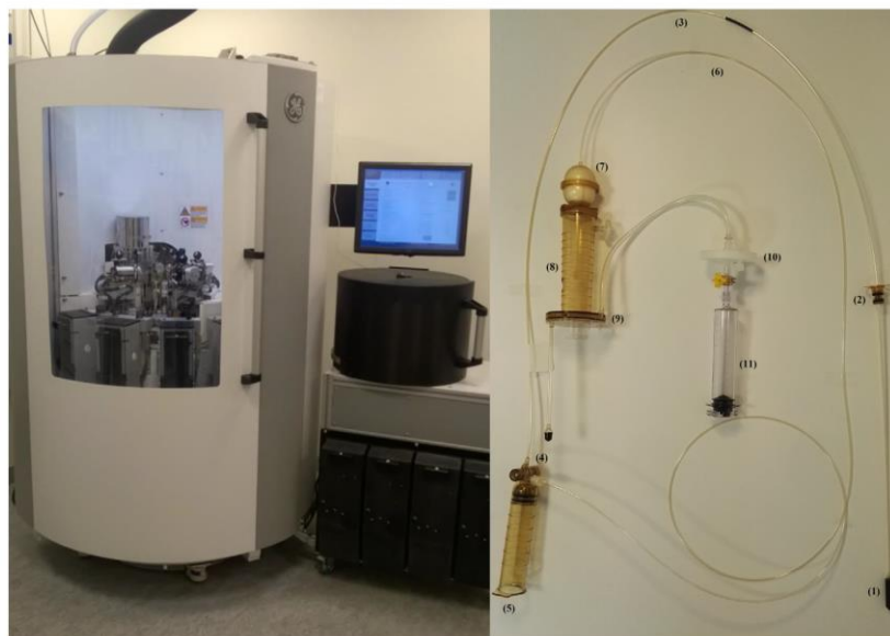
Fig. 1. (A) SPINlab polarizer. The polarizer operates at 5 T and 0.9 K [16]. The polarizer has four independent channels that allow simultaneous polarization of up to four samples (fluid paths). The QC module (cylindrical black unit) is seen to the right of the photo below the touch screen. (B) Fluid Path (FP). Part A: (1) vial, (2) dynamic seal, (3) co-axial tube, (4) valve, (5) dissolution syringe. Part B: (6) transfer tube, (7) EPA filter, (8) receiver vessel, (9) QC appendage, (10) sterile assurance filter, (11) Medrad 65 mL MR syringe. Part A loads into the polarizer (behind the sliding door). The vial is inserted into one of the four airlock and the dissolution syringe is inserted into the corresponding heater-pressure module. After some pump-flush cycles, the airlock gate-valve will open and the vial can be pushed through the dynamic seal to the 0.9 K sample space. Part B is initially loaded into the corresponding warmer module seen to the lower right in (A). Shortly before dissolution part B is moved from the warmer to the QC module.
