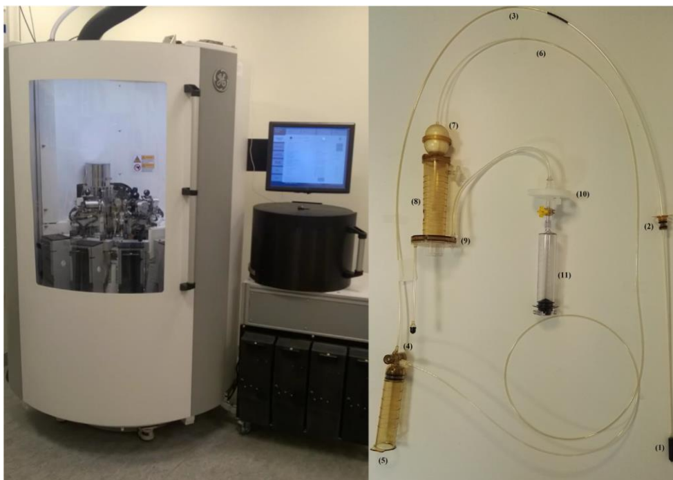
Figure 4 – Left: GE SPINlab polarizer, operating at 5 T and 0.9 K. The polarizer is equipped with four independent channels able to accommodate four samples (fluid paths) simultaneously. The cylindrical black unit is the quality control (QC) module, capable of measuring relevant parameters for the product (post dissolution), before the sample is released and injected into the subject. Right: Fluid path. The sample is sealed in a vial and the dissolution media is placed separately in a dissolution syringe, which is loaded into the SPINlab polarizer. Adapted from Malinowski et al. (Paper III).
