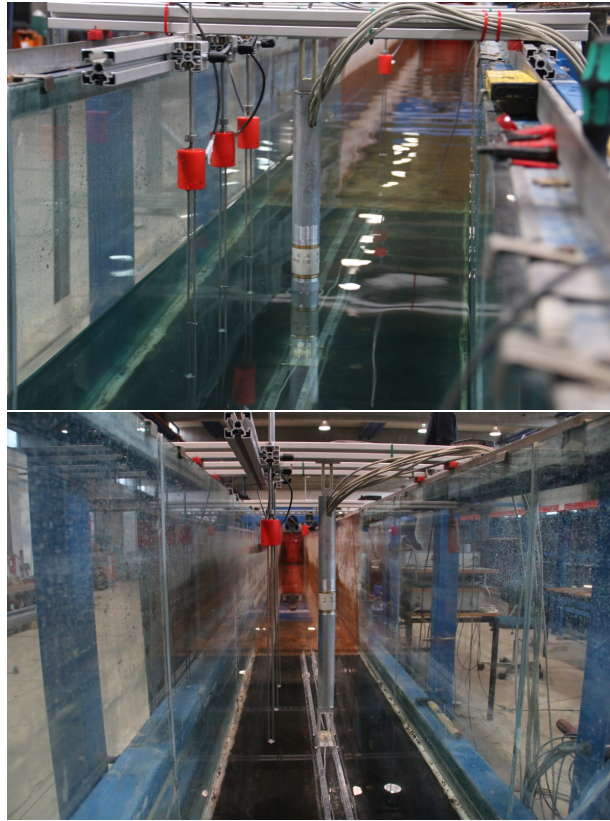
Figure 6.2: Arrangement of cylinder and wave gauges WG1, WG2, WG3 and WG4 in the experiment.
