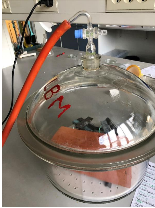
Figure 4: Brick and mortar sample in a desiccator during the density and porosity tests
