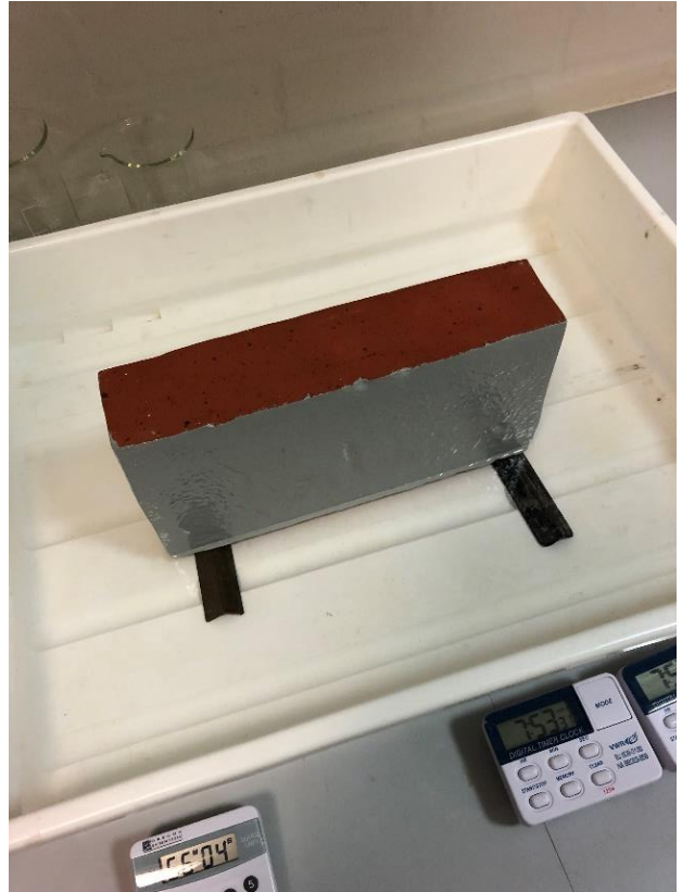
Figure 6: Partial immersion test of the historic brick with the exterior surface facing the water and sealed with epoxy on the four sides
