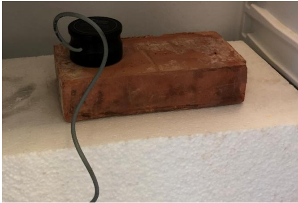
Figure 2: Surface probe placed on the bricks surface
