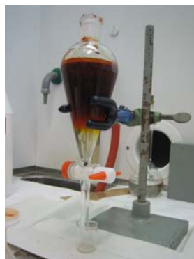
Fig 1. Mineral separation with \text{CCl}_4 .
