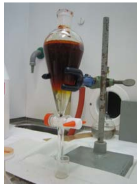
Fig 1. Mineral separation with \text{CCl}_4 .
