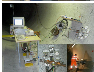
Figure 2. In situ experiment site located in the WT tunnel of the GTS. The length of the injection borehole was 1.27 m, diameter 4 cm. Overcoring was performed with a 300 mm single core barrel which provided an intact drillcore (PSG 04.001-OC) of 1.17 m length.
