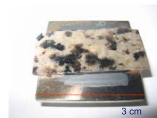
Figure 2. A SEM sample of the El Berrocal granite.
