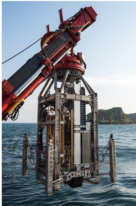
Figure 2.9: The BGS RD2 System being deployed using dedicated Launch and recovery system
