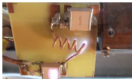
Figure 2. Photograph of electrical discharge in low pressure helium atmosphere across matching network components during transmit pulse.
