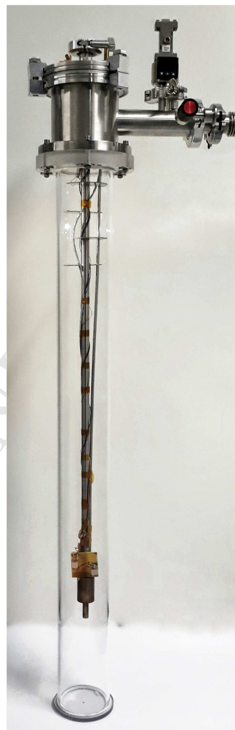
Figure 15. Photograph of the transparent plastic chamber for electrical discharge testing. On top the adapter for probe and pump connection is seen. The probe is inserted in the chamber.
