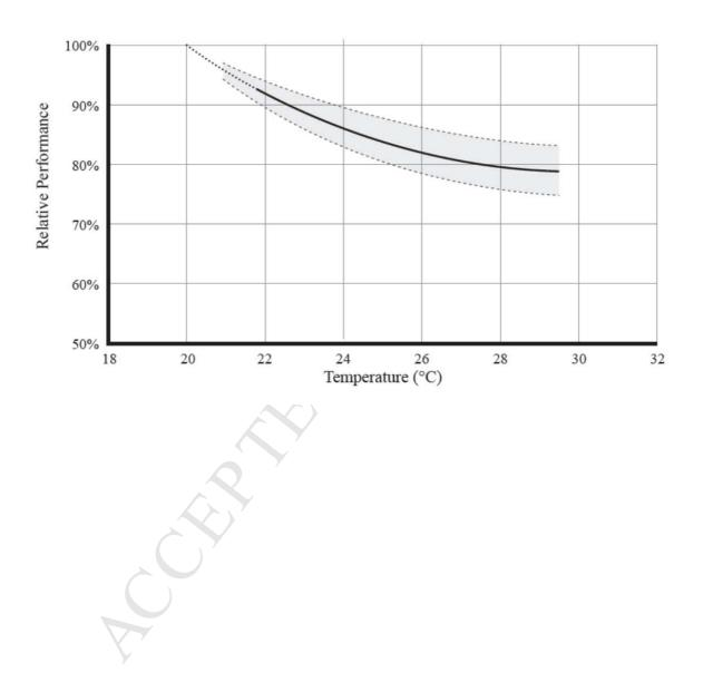
**FIGURE 3.** Comparison of the relationship developed in this study with the relationships proposed by Auliciems [12], Wargocki and Wyon [2], Seppänen et al.[18], and Lan et al.[22]. Dashed lines show relationships for schoolwork while continuous lines for adults doing mostly office work. Optimal conditions for performance are considered to occur when performance is 100%. The details of these relationships can be found in the supplementary material Table A3.
