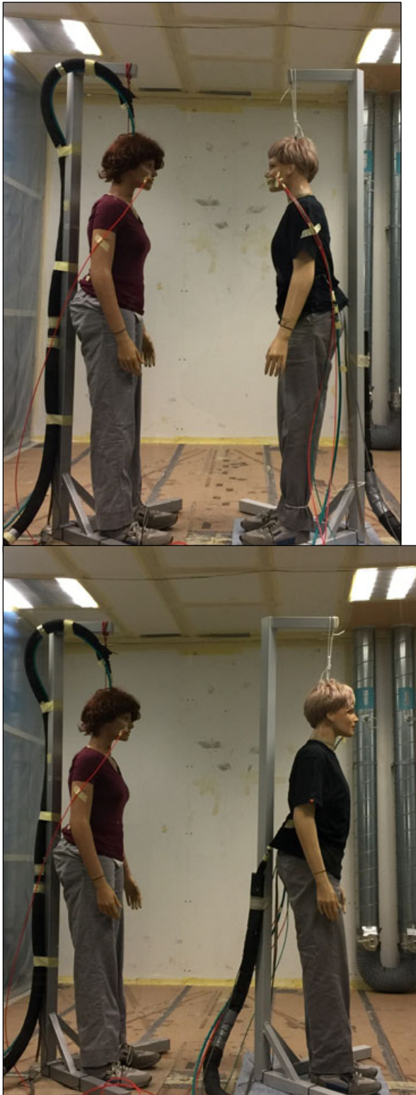
Figure 2 The real-life set-up of the face-to-face (Termed Positioning A) and face-to-back positioning (Termed Positioning C), in which the left manikin simulated an infected person and the right one an exposed person; the tubes visible in the figures were used for connecting the artificial lungs and tracer gas monitors.
