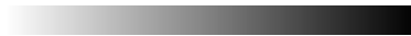
Figure 2: Gray scale employed to represent topologies. White represents the void phase ( \bar{\rho} = 0 ) and black the solid phase ( \bar{\rho} = 1 ).
