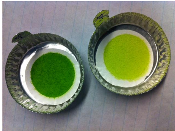
Figure S6: Colour change due to nutrient limited conditions (see Fig. 2a). The left metal plate contains a glass-fibre filter that has a deep green colour, due to high chlorophyll content at nutrients in excess conditions (see Fig. 2b). The metal plate on the right contains a filter that has yellowish colour due to the increase in carotenoid level under nutrient limited conditions.
