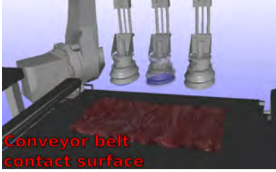
Fig. 13: A planar constraint is used to ensure the meat does not fall through the conveyor belt.
