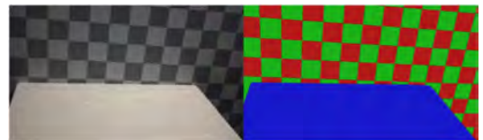
Fig. 6. Labeling of the image to the left results in the label image to the right. Each color in the label image represents a label that we assign a BRDF to. The black edges between labels indicate areas where we apply a nearest neighbor method.
