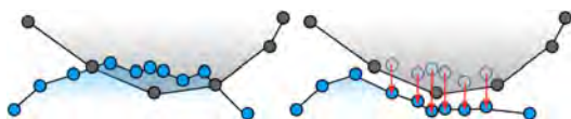
Fig. 8. Deformation of background mesh, where we push the background vertices down to avoid mesh intersection.
