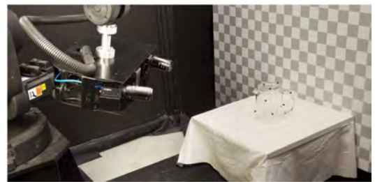
Fig. 13. Scene with checkerboard backdrop, lighting, glass teapot, and stand with table cloth observed by two cameras mounted on a 6-axis industrial robot arm.
