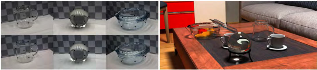
Fig. 1. To the left, we compare rendered images (top) with photographs (bottom). More views are available in Appendix A. The scenes to the left were digitized using our pipeline and include both glass objects and non-transparent objects (tablecloth and backdrop). To the right, we exemplify the use of our pipeline for virtual product placement using our digitized glass objects, with estimated optical properties and artifact-reduced removal of markers.
