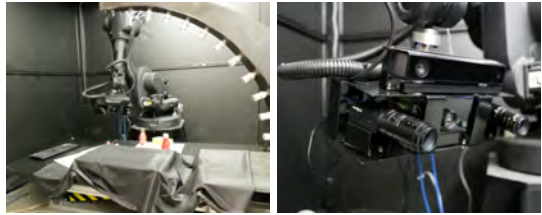
Fig. 1. Mobile structured light scanner used to acquire 3D data for the data set.
