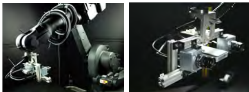
Figure 1. Photos of the 6-axis industrial robot mounted with two cameras and a projector. Cameras allow for MVS, and in conjunction with the projector SL provides ground truth point clouds.
