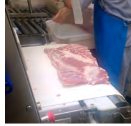
Fig. 10: Human meat placement. The meat is placed on the conveyor belt with a flat front facing the wrapping station.
