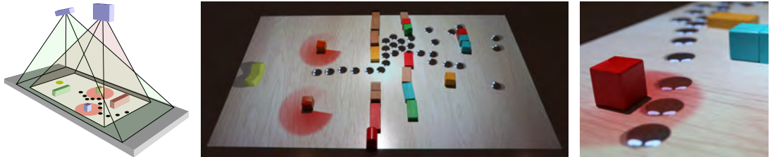
Figure 1: (left) Our setup using projector (red frustum) and a Kinect camera (green frustum). (middle, right) Pictures of the gameplay.
