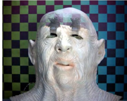
Figure 6. Actuators for manipulating the geometry of the mask. The image of the mask has been superimposed on an image of the actuators, illustrating their functionality.
