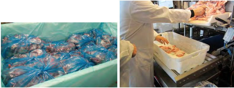
Figure 1.1: The practical use case for this thesis. The deceptively simple process of picking meat from an unorganized pile (left) and placing it on e.g. a conveyor belt.
