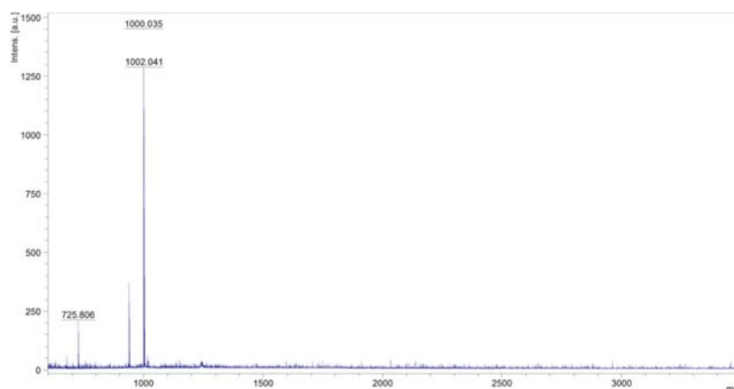
Figure 2.6 Mass spectra of Cu-PC complex. The peak of 1000 presents the mass of [\text{PC-Cu}]^+ complex. The peak of 1002 presents the mass of PC-Cu complex + H.
