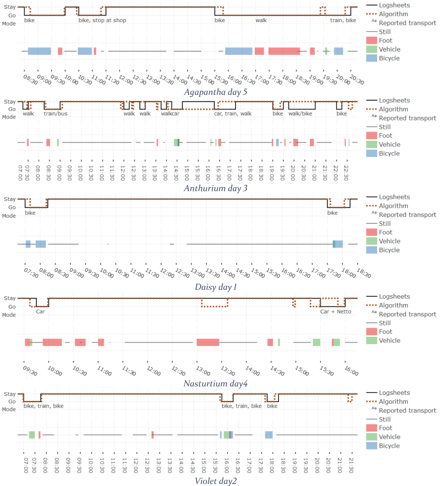
Figure 14. Time charts comparing log sheets and algorithm results for trajectory extraction and activity bout detection. A single day from each participant is shown.
