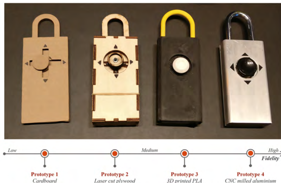
Figure 1. Photograph of the four prototypes of the padlock design used for the study; The process bar in the bottom illustrates how the fidelity of the prototypes increases from left to right
