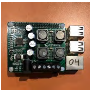
Stack of Raspberry Pi and HiFi Berry Class-D Amplifier
