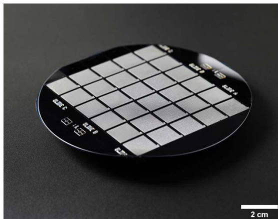
Figure 8 – Picture showing a Si wafer with MCs distributed in an array of 5x6 chips of 25x25 MCs.
