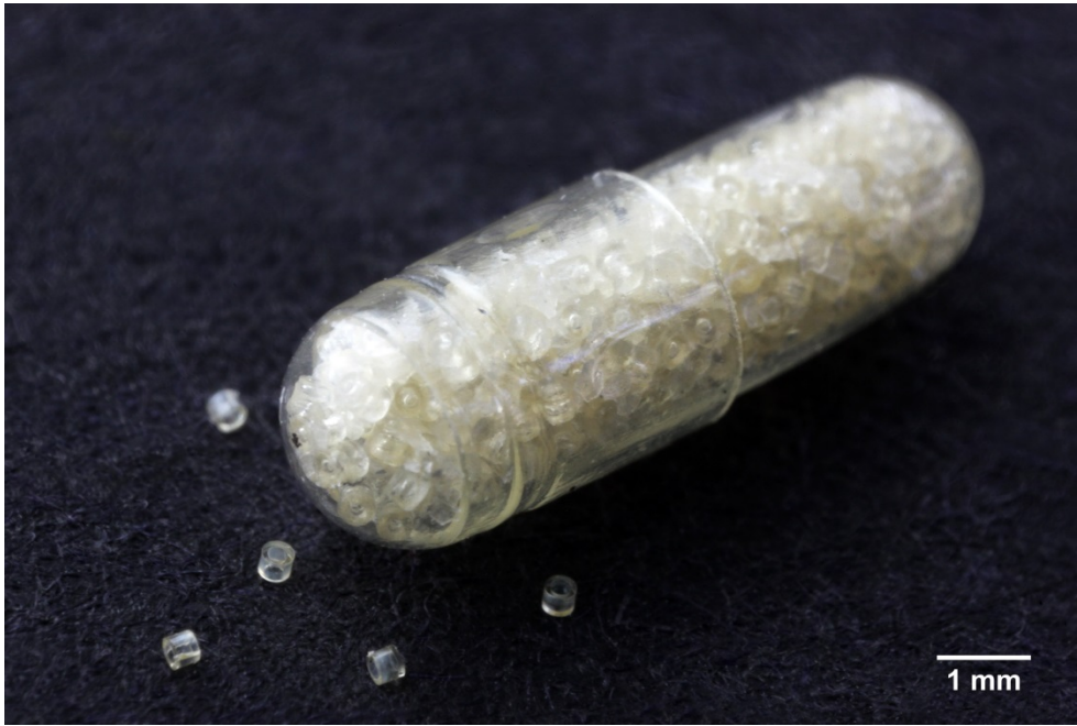
Figure S5: Picture of a gelatin capsule filled with loaded and coated D-MCs. Empty D-MCs are positioned outside the capsule for comparison.
