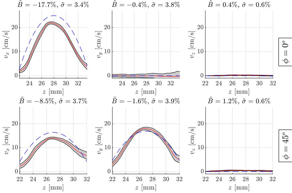
Fig. 2. Parabolic flow profiles, measured on a constant flow rig (setup 1) with  $v_{peak} = 0.25$  m/s. In total 10 estimates were averaged to reveal a single profile. The estimated profile is shown in red, the shaded gray area show plus minus one standard deviation, and the dashed blue line is the true profile. The top panel has a rotation of  $0^\circ$  around the  $z$ -axis. Bottom panel a rotation of  $45^\circ$ .
