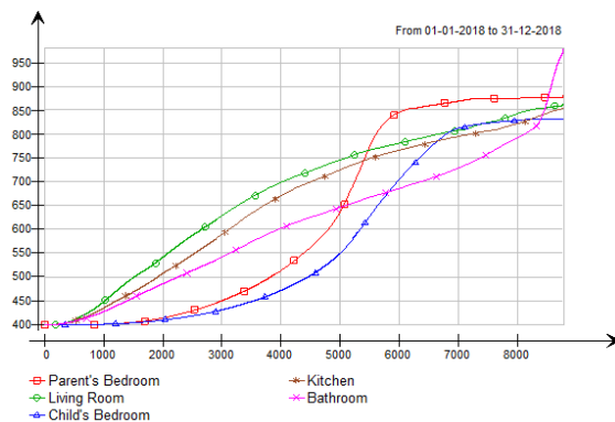
Figure 3. Duration curve of CO 2 concentrations with room-based demand-control.
