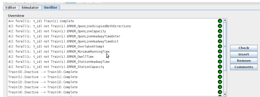
Fig. 4. Verification results for the timetable for Nærumbanen in Denmark.
