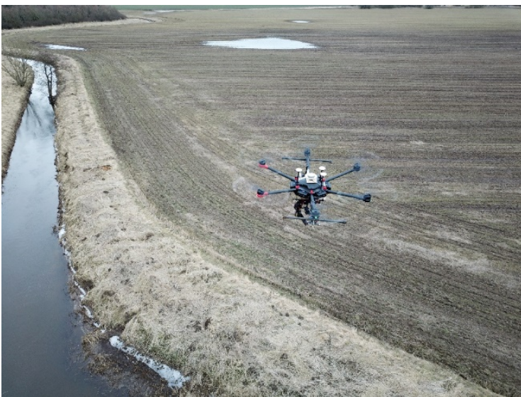
270 Fig. 6, UAV flight to retrieve WSE observations in Åmose Å, Denmark.
