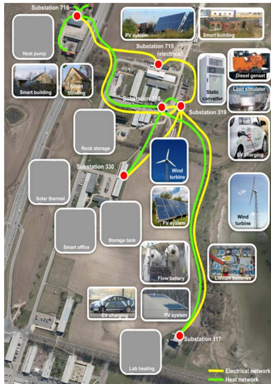
Figure 5. Lay-out and details of PowerLabDK/SYSLAB
