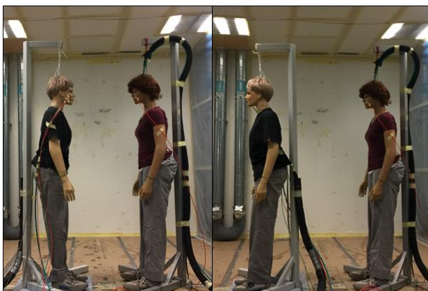
Fig. 2. Views of experimental set up, the manikins are placed face-to-face and face-to-back
