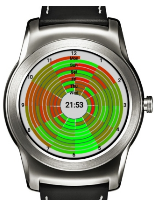
Figure 2: Data visualization using a time spiral on a 12 hour analogue clock face. Each hour is color-coded green-red to indicate number of data points or severity of the observations (e.g. of a symptom)
