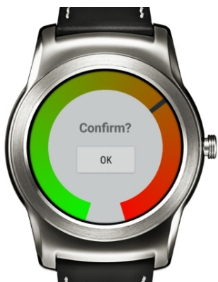
Figure 1: A Visual Analogue Scale (VAS) mapped onto the edge of an analogue clock face. This way the scale has a length of 9.8cm close to the standard 10cm VAS
