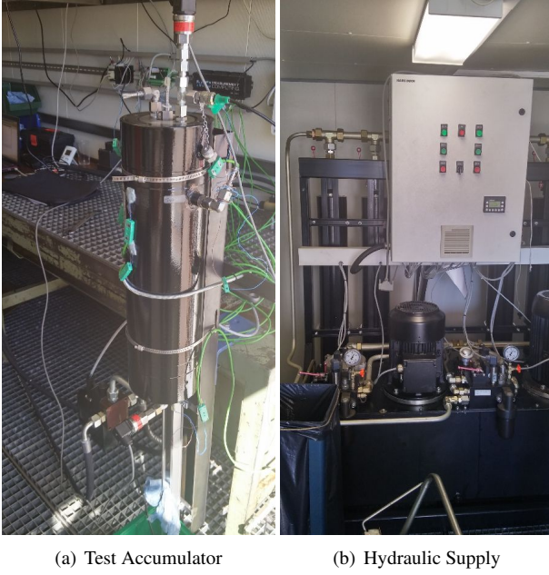
Figure 6: Main hydraulic components of the experimental rig
