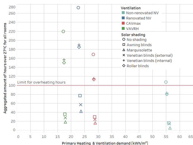
Fig. 7. Yearly primary energy use and number of occupied hours with indoor temperature over 27 °C in the apartment oriented towards west for cases without the surrounding buildings.
