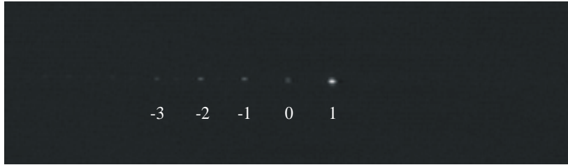
Fig. 5. Diffraction from a linear blazed grating encoded on the SLM. The experimentally obtained diffraction orders are labeled as -3, -2, -1, 0, and 1, respectively.
