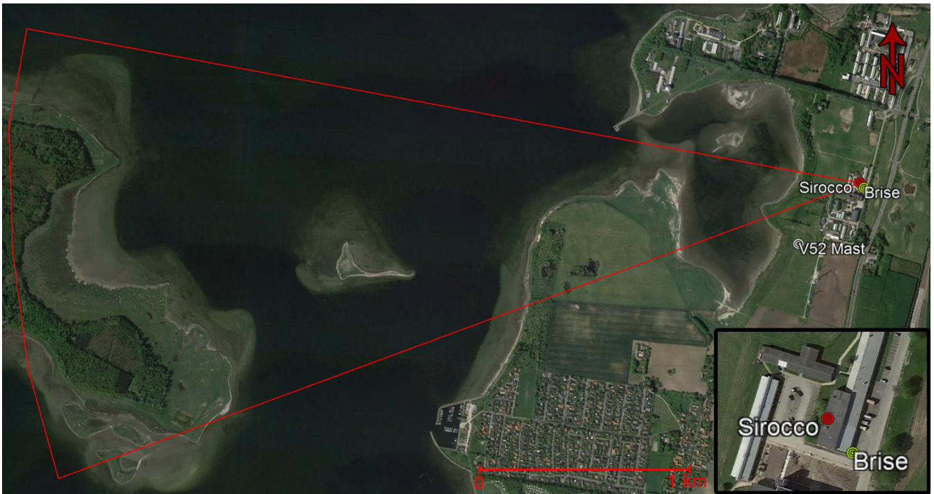
Figure 3. LASCAR experiment overview, with positions of the two scanning lidars and the met-mast denoted. The radius of the arc is 4 km
