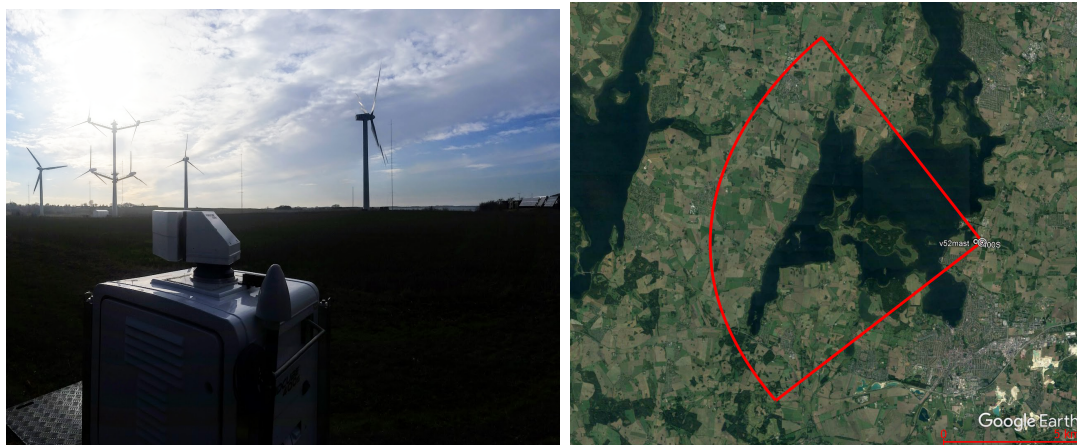
Figure 3.1: Left: Photo of scanning lidar taken during experiment. Right: Aerial view of measurement setup. The radius of the arc is 9.6 km.
