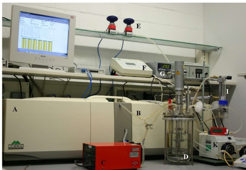
Figure 13: Bioreactor system with in-line laser diffraction analysis; A Malvern MasterSizer 2000, B bypass, C peristaltic pump for bypass, D 3 L bioreactor, E off-gas analysis, F pH regulator, G temperature regulator, H stirrer regulator, I rotameter for air flow control, J thermal mass flow meter for air flow check-up, K dosing pumps for pH adjustment
