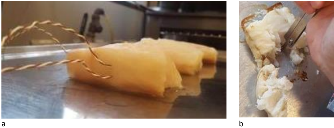
Figure 4 Measurements of the core and surface temperature. a) The probes inserted into the loins before baking. b) Registering the position of the temperature probes after baking using a caliper.
