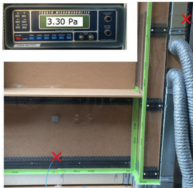
Figure 52: Pressure drop measurement of mock-up model
