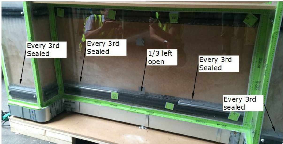
Figure 49: Sealed perforations to force air to flow beneath window
