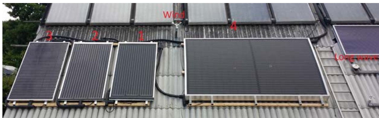
Figure 1. The prototype collectors tested. They are connected in series and have the same flow rate. The collector size is 2 m 2 respective 6 m 2 .
