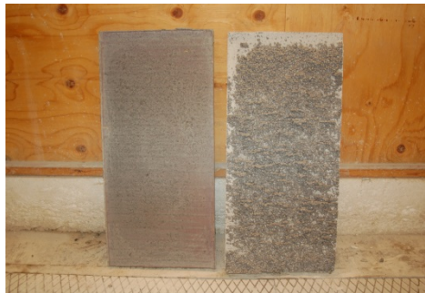
Figure 5.6. Typical HPC faces of push-off test specimens after failure.
