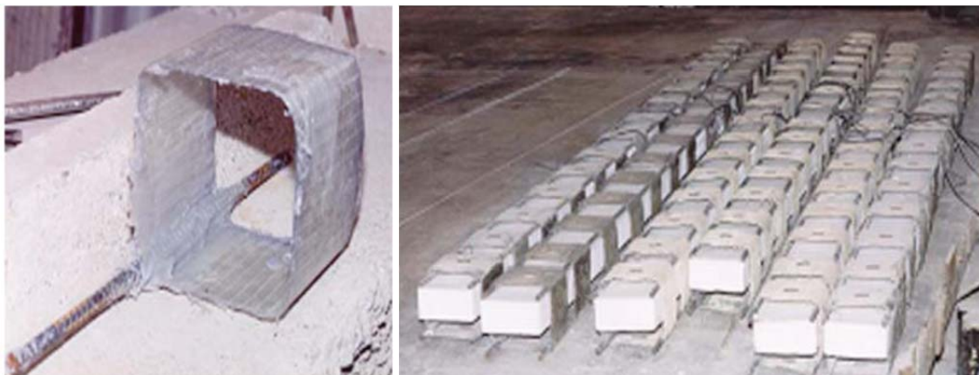
Figure 1.5 Photo of GFRP Shell with reinforcement and foam insulation installed (Pantelides et al., 2008).
